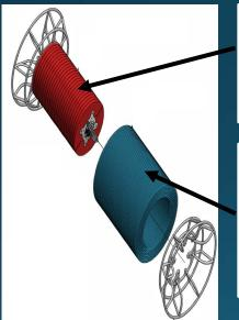
Low-Density Syntactic Foam (450m operational depth); >180lb buoyancy
