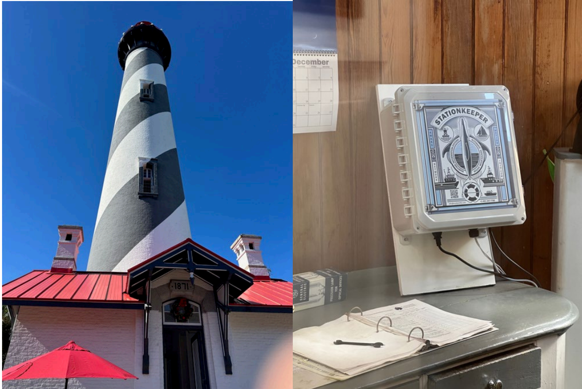
An AIS installation installed at the top of the St. Augustine lighthouse. Messages advising of over speed and avoidance are sent to vessels within a 20-mile range, and acknowledgement of the message received. (Photos: T. McGinis).
